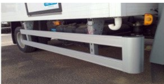
Figure 2: Side under-run protection
