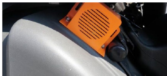
Figure 6: Vehicle manoeuvring warning for left-turning
