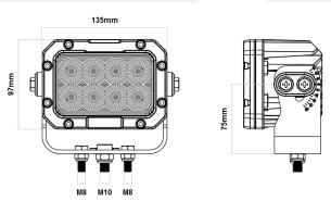
These ultra-high-powered industrial flood work lights use the latest LED technology to maximise the luminosity output resulting in a light that will cover a huge area even in pitch black conditions. Multi-voltage, ECE R10 approved and rated to CISPR 25 Class 4 - this light is the ideal choice for industrial applications. Available with 8-LEDs emitting 6400 lumens, or 12-LEDs emitting 10,200 lumens.
