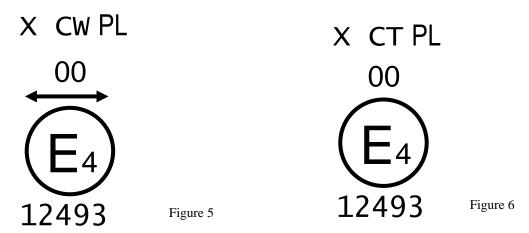
The installation unit, bearing the above approval mark is incorporating a lens of plastic material and meeting the requirements of this Regulation in respect of the passing-beam only and is designed:
