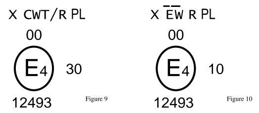
Figure 9: In respect to the Class C passing-beam, the Class W passing-beam both with bending modes and a driving-beam, and designed for right-hand traffic only.
