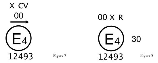
Figure 7: The installation unit, bearing this approval mark is meeting the requirements of this Regulation in respect of the Class C passing-beam with Class V passing-beam and designed for left-hand traffic only.
