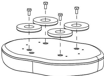
Four magnets are fixed with 4 screws at the bottom of the lightbar
