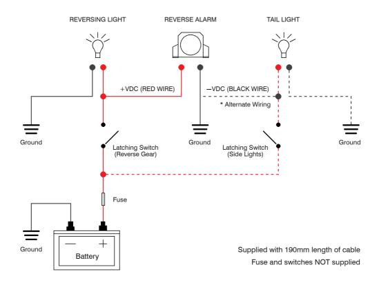
\* ALTERNATE WIRING FOR NIGHT SILENT FUNCTIONALITY - Connect the Reverse Alarm —VDC (BLACK WIRE) to the Tail Light +VDC (RED WIRE). Otherwise, connect the —VDC to Ground to use the alarm at all times of the day.
