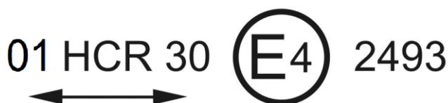
The headlamp bearing the above approval mark meets the requirements of this Regulation in respect of both the passing-beam and the driving-beam and is designed:
