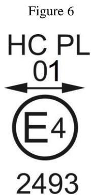
The headlamp bearing the above approval mark is a headlamp incorporating a lens of plastic material meeting the requirements of this Regulation in respect of the passing-beam only and is designed:
