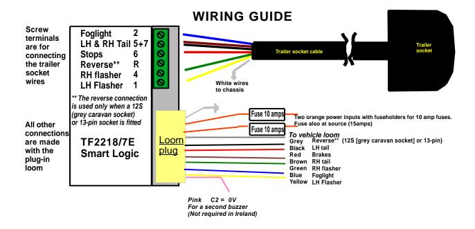
How to connect if you use a single power cable through the vehicle
