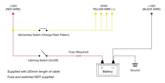
TO CHANGE FLASH PATTERNS - Momentarily apply yellow wire to the +VDC. A simple momentary switch will be sufficient.
