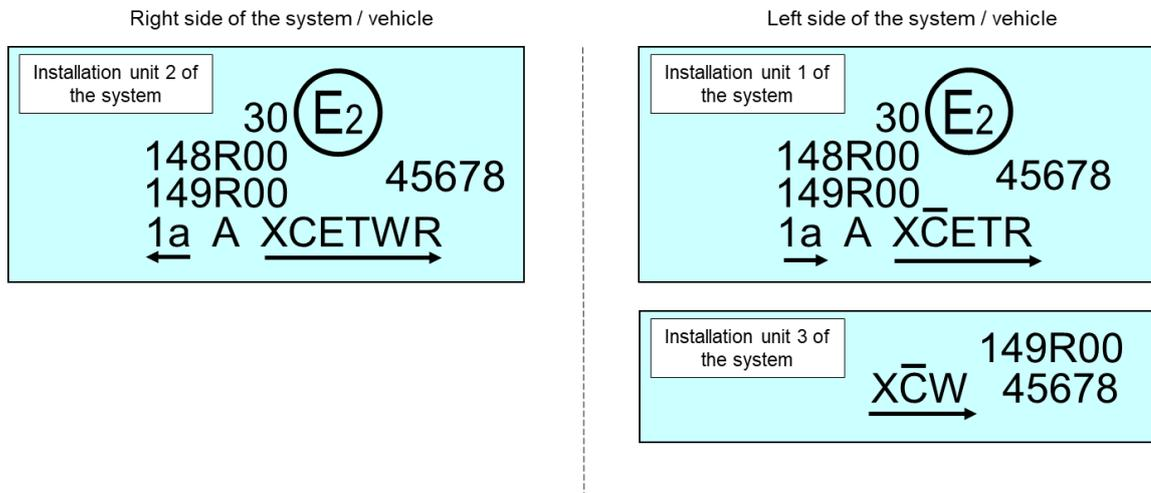
The system bearing the above approval markings meets the requirements of this Regulation (original version of the Regulation) in respect of both a passing-beam for left-hand traffic and a driving-beam with a maximum intensity comprised between 123,625 and 145,125 candelas (as indicated by the number 30) grouped with a front direction indicator lamp of category 1a and a front position lamp approved in accordance with the 00 series of amendments of UN Regulation No. 148.
