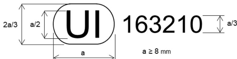
The above Unique Identifier marked on the lamp shows that the type concerned has been approved and that the relevant information on that type approval can be accessed on the UN secure internet database by using 163210 as the Unique Identifier.
