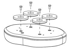
Four magnets are fixed with 4 screws at the bottom of the lightbar
