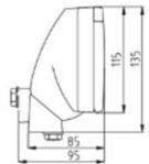
ABL Beta X3M is a full beam work light built to the most stringent quality demands. It is equipped with a HID bulb (Xenon). HID Xenon delivers three times the light compared to the traditional halogen bulb, at less power consumption (35W). The service life of the bulb is about ten times compared with a halogen one (55W). Beta X3M is also more withstanding to vibration and gives a light that is more similar to daylight.
